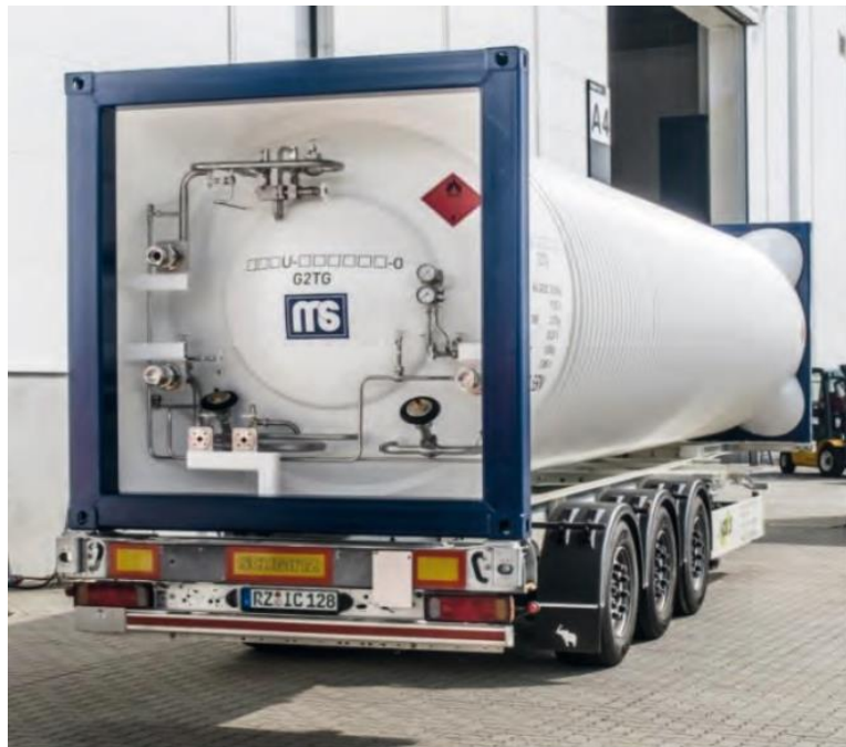
Fig 10. Container with marine LNG fuel block [11]
