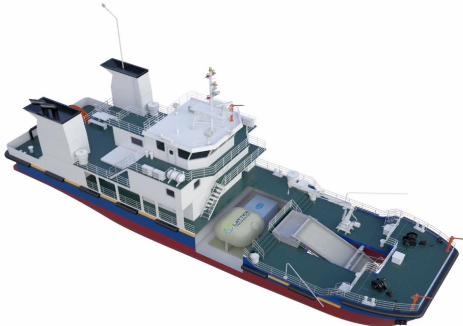
Fig 23. LNG fuelled port cleaning ship [21]
