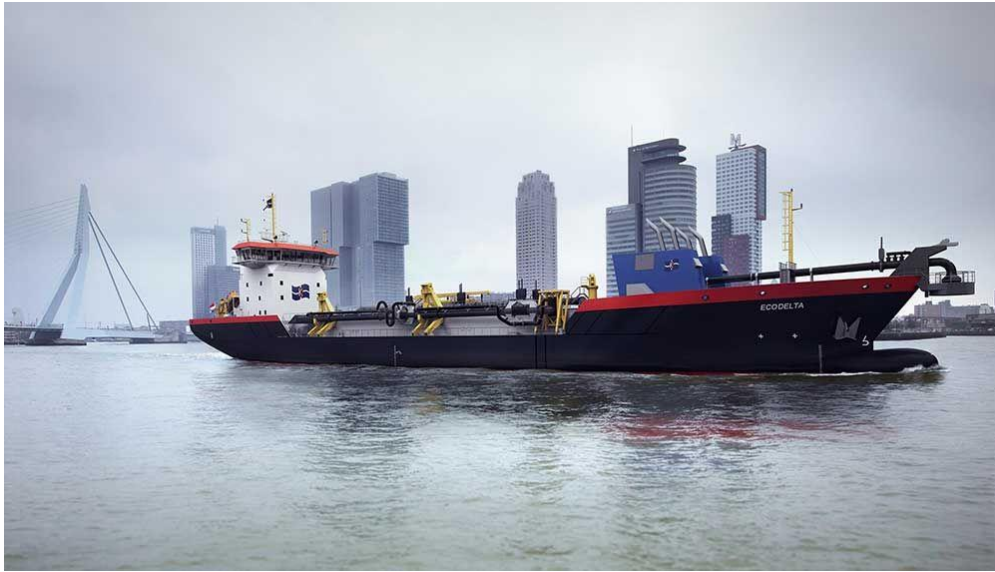
Fig 24. LNG-powered dredging vessel [22]
