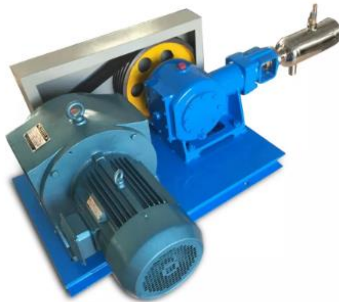
Figure 9. Low-pressure cryogenic pump [19]
