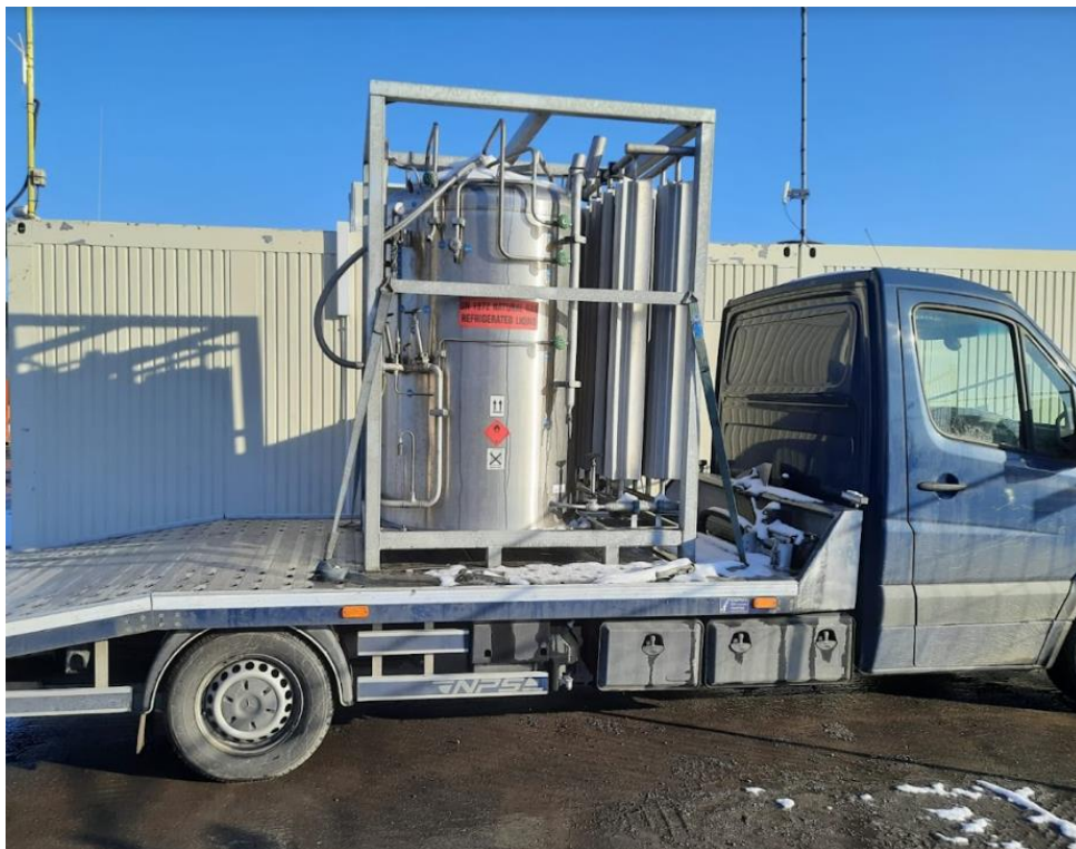
Figure 11. Cryogenic tank (mini-tank) for the transport of bioLNG / LNG - Microfueller LNG (own materials)
