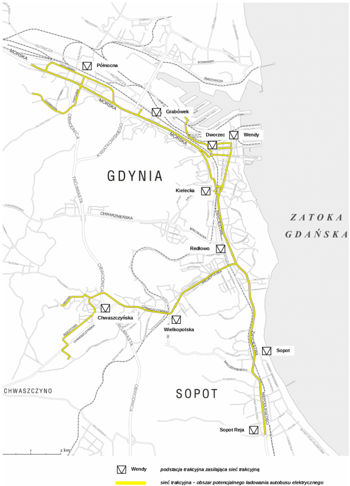
Figure 3. The map of the traction network with the distribution of supply substations [9]
