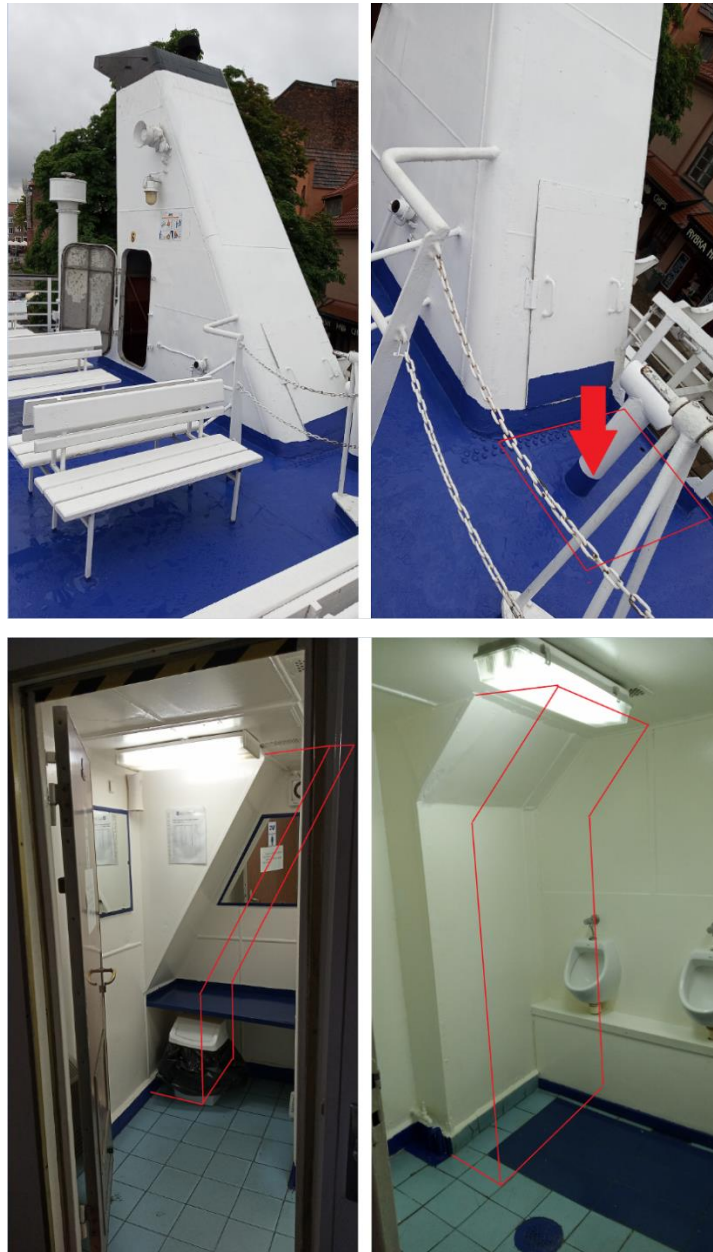
Figure 32. A proposal of a deck penetration with a gas pipe and cooling water (supply + return) and marking a new shaft along the existing one on passenger decks.
